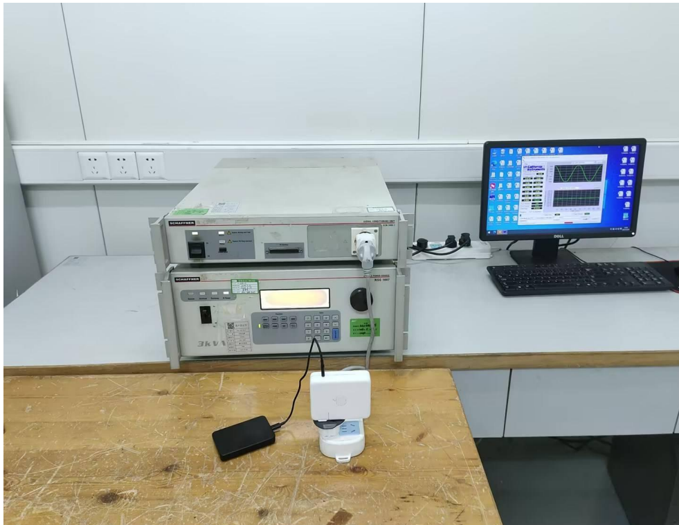
Harmonic current emissions & Voltage fluctuations and flicker
