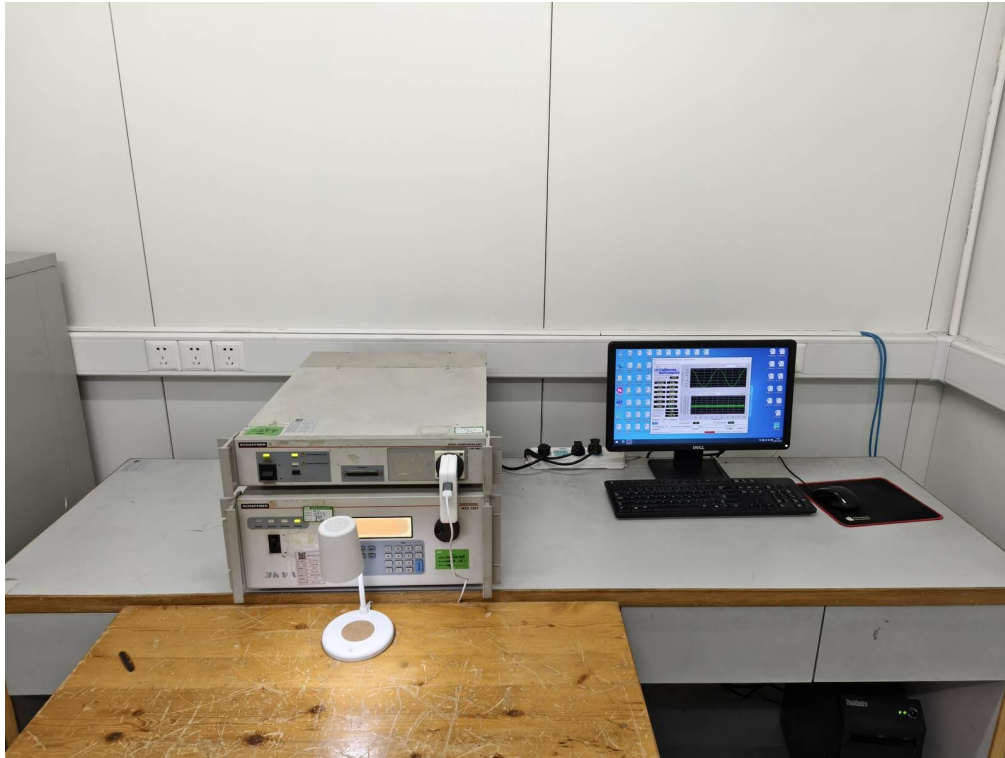
Harmonic current emissions & Voltage fluctuations and flicker
