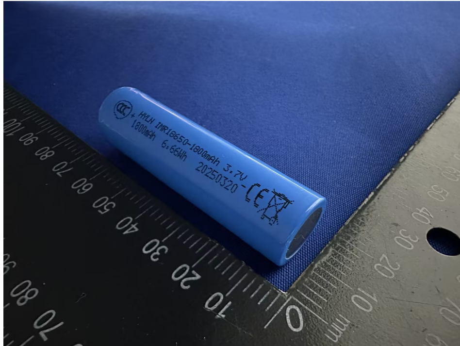
Picture 7. Side view-1 of cell for model HYLN IMR18650-1800mAh
