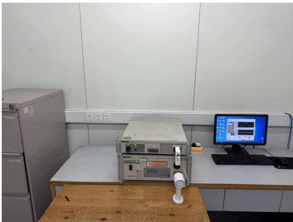
Harmonic current emissions & Voltage fluctuations and flicker
