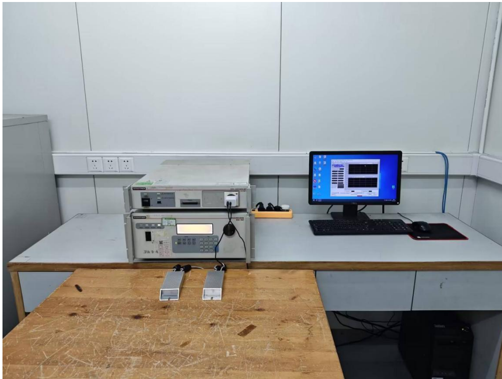
Harmonic current emissions & Voltage fluctuations and flicker
